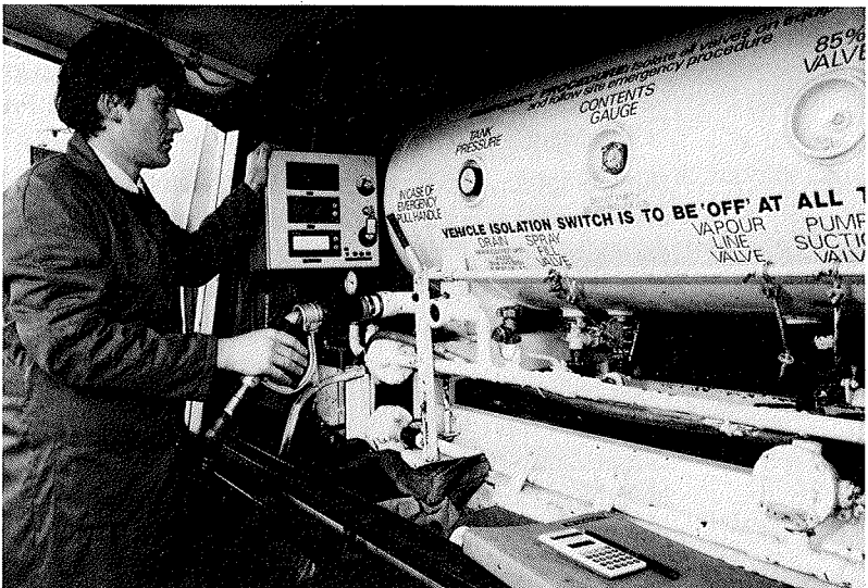
Ken Millis of the Inspection Services checks an LPG dispenser at a service station for accuracy. Thirty-one per cent of gas dispensers so far tested did not meet the required tolerances for accuracy.
