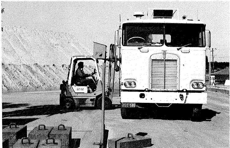
A fork-lift unloads 500kg weights from the Weights & Measures truck to ensure the accuracy of a weighbridge.
